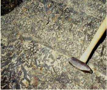
In a rock, hornblende visit http://www.pitt.edu/ If you can remember that the amphiboles from oblique cleavage planes of approximately 120 degrees, whereas pyroxenes have cleavage planes of approximately 90 degrees it will surely help you decide between the two. Amphiboles also are specifically less dense than their corresponding pyroxenes. Hope this helps you.
