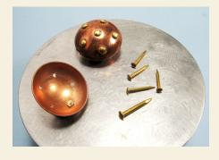
Be sure to get solid brass pins, not brass plated steel. If unsure, test them with a magnet.
