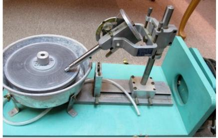
29. "Exacta Faceting Machine" by Franz Eisele, a Mast Type Faceting Machine. This may be one of the last simple Mast designs that has no number-keeping for reproducing the mast height of the Coarse Facets for Fine-Grinding and Polishing. After setting the coarse height by touching the stone to a non-rotating Lap, the *initial* Height Setting is <u>re-located</u> on a slowly rotating Lap for the Fine-Grinding and Polishing by making shallow trial cuts.
