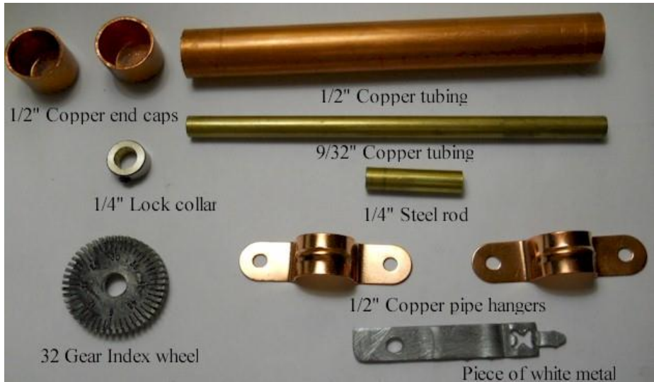
57. "Merlyn". The parts for a Homemade build it yourself faceting head.
