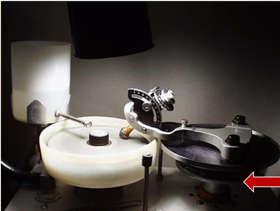
22. “Raytec Shaw.” A Removable Hand piece Faceting Machine. Underneath the Hand piece and Table, a Rotating Ring raises or lowers the Table for the Coarse Height Adjustment to cut different Angles.
