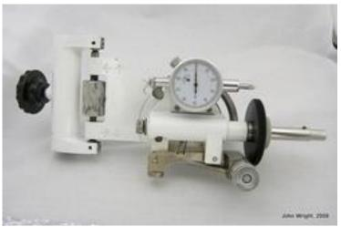
36. A "Graves" Faceting Head with an aftermarket Dial Indicator to minimize the Mast Flex problem. In many applications, a *Non-Spring-Loaded Dial Indicator* will release all of the Flex of the Mast but may still allow any loose bearings to wobble.
