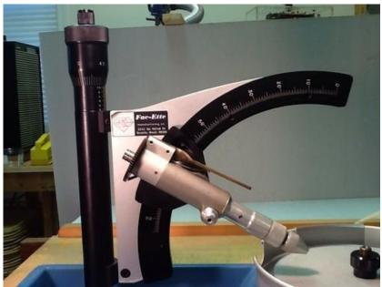
39. "Fac-Ette" – A Mast Type Faceting Machine. The very large and *easily read* Protractor has enough weight on one side of the Mast to reduce Tube-on-Mast Bearing Wobble. Note that even this Protractor reads to half of a degree, estimated to a tenth of a degree
