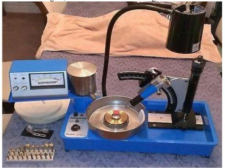
40. "Fac-Ette GemMaster" an improved "Fac-Ette" with an *electronic* **Strain Gauge** to *eliminate* the Mast Flex problem. This is <u>the *first successful*</u> **Depth of Cut Indicator**. Cut until the needle reaches the green band on the meter; stop before hitting the red band. Repeat for subsequent facets. Movement of the needle shows the speed and progress of the cutting.
