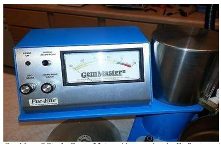
41. The "Fac-Ette GemMaster" **Strain Gauge Meter** with a warning **Audio System.** An alarm sounds after just passing the green band at Zero.
