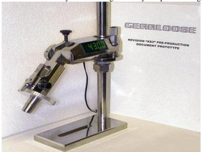
49. "XS 3". Jonathan Rolfe, a.k.a. 'Gearloose', Mast Type Faceting Head with an Electronic Digital Protractor. It is made from made from non-flexing Titanium to "eliminate" Mast Flex. Rolfe published build-it-yourself instructions in Lapidary Journal before he made 78 copies for the Graves Company sold as the "Graves Mark V XL".
