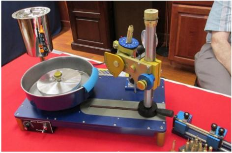
51. "Jersey Instrument". A Mast Type Faceting Machine. One of the newest, very robust faceting machines; the design originated in Australia. Note the **Direction of Rotation Control** and the variable **Speed Control**, features found on most electric powered faceting machines. Some gems have "grain" that makes polishing certain facets difficult. Changing the direction of rotation during the polishing of a facet sometimes diminishes the problem.
