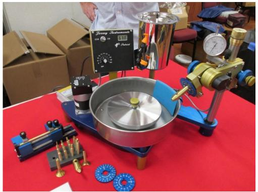
53. "Omni-E" by Jersey Instruments. A Mast Type Faceting Machine with No Slide Base. This is the second faceting machine by Jersey Instruments. Jersey Instruments purchased the design from Laurie Hall and made modifications.
