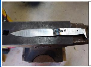
Here are some pictures of what I have been doing. First is a knife that I made from a railroad spike. And below is a stone that I have cut from some uranium glass. It fluoresces, as you can imagine, green. I have now moved on to forge a dagger from a truck leaf spring and to real stones.
