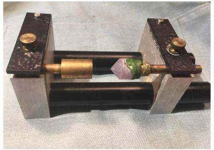
Other brands: I would rotate the dop slightly while moving the stone towards the next dop with Epoxy. Assure yourself by the feel that there is no high spot on a dop resting in a "V" grove. Good luck with the dops-in-the-chuck-alignment if you have damaged dops.
