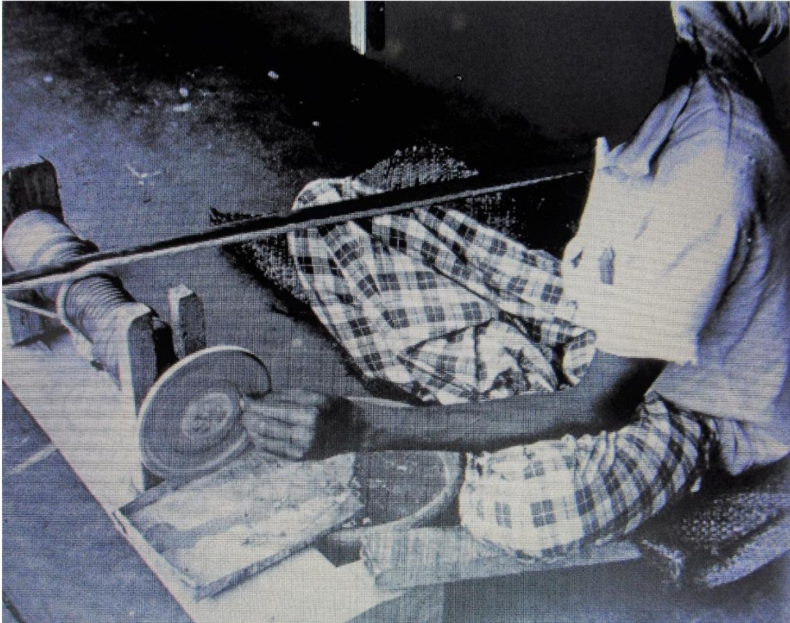
2. Another **Hand Powered**, Hand Faceting example. Move the bow one way for rotation; slack and return the bow to the starting position. The heavy Spindle acts as a flywheel maintaining the spinning momentum.
