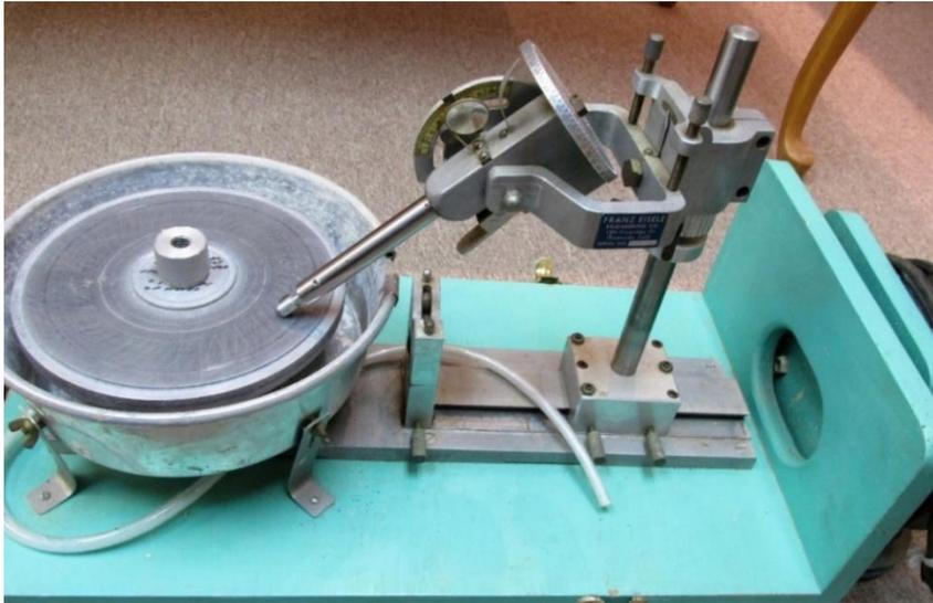
29. “Exacta Faceting Machine” by Franz Eisele, a Mast Type Faceting Machine. This may be one of the last simple Mast designs that has no number-keeping for reproducing the mast height of the Coarse Facets for Fine-Grinding and Polishing. After setting the coarse height by touching the stone to a non-rotating Lap, the *initial* Height Setting is re-located on a slowly rotating Lap for the Fine-Grinding and Polishing by making shallow trial cuts.
