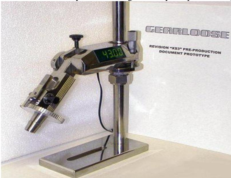
49. “XS 3”. Jonathan Rolfe, a.k.a. ‘Gearloose’, Mast Type Faceting Head with an Electronic Digital Protractor. It is made from made from non-flexing Titanium to “eliminate” Mast Flex. Rolfe published build-it-yourself instructions in Lapidary Journal before he made 78 copies for the Graves Company sold as the “Graves Mark V XL”.
