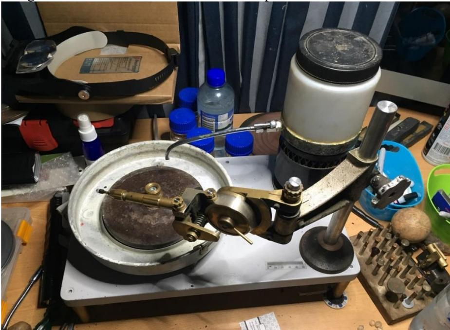
52. “Hall”. An early Laurie Hall Mast Type Faceting Machine from Australia with **No Slide Base**. A second arm allows faceting in the “working area” of the Lap as the Height is changed. (See #26.) Hall made a number of improvements to faceting machines and a number of unique well-liked machine designs although reportedly, he never cut a gem.
