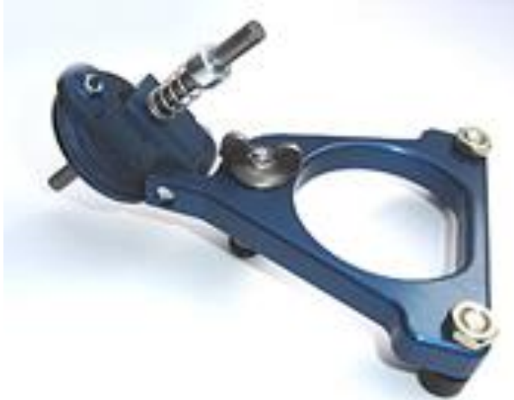
62. “Tes Lap”. A hand Powered, Movable Handpiece ; no Spindle and Lap. Is it a “Jack Lear” spin-off, or is it a “Raytec” imitation? Note the Radial Adjustments and Fine Height Control. Moving the Dop/Quill in or out is the Coarse Height Control. Use a handheld Protractor to set the Angle on these Movable Handpieces.
