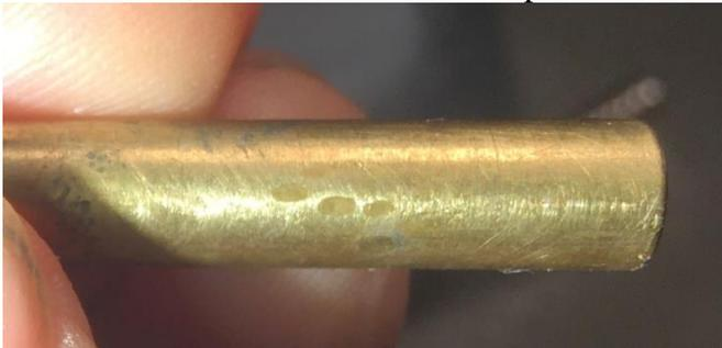
Careful: do not change the diameter or roundness of the dop shaft. This “cure” allows me to facet to near perfection. Be sure the dops are clean of any wax film or crud along the shaft: clean with alcohol.
